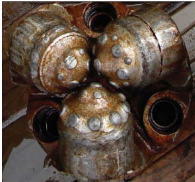
These photos were taken after drilling the Nikanassin section. In Fig. 8a, the bit drilled from 1,356 m to 1,683 m through the Nikanassin and was graded as 6-6-FC-A-E-3-FC-HR. In Fig. 8b, the bit drilled from 1,683 m to 1,895 m and was graded as 8-8-SD-A-F-30-CC-PR (Fig. 8).
