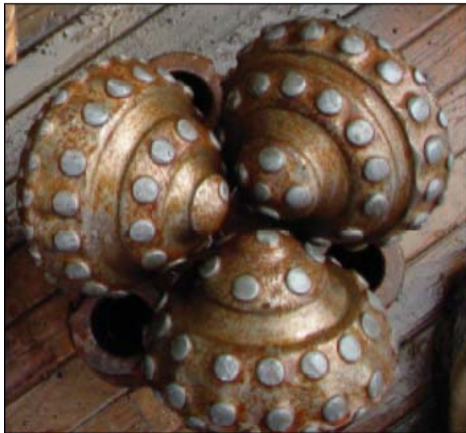
These photos were taken after drilling the Nikanassin section. In Fig. 8a, the bit drilled from 1,356 m to 1,683 m through the Nikanassin and was graded as 6-6-FC-A-E-3-FC-HR. In Fig. 8b, the bit drilled from 1,683 m to 1,895 m and was graded as 8-8-SD-A-F-30-CC-PR (Fig. 8).
